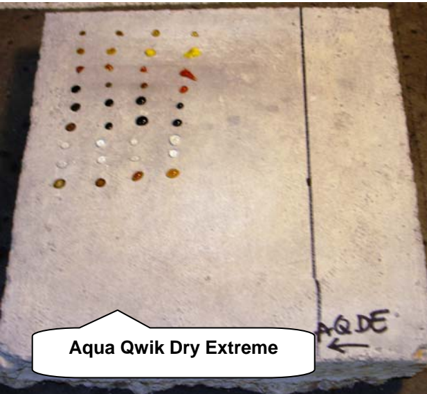
Steel Troweled Concrete With Stains Applied
